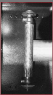
Applegate Industrial Materials manufactures a complete line of braided connectors for both vibration control and misalignment compensation. Stainless steel annular corrugated flex inside of a layer of stainless steel woven braid, all welded into a strong, leak tight assembly. Each hose assembly individually tested to 150 P.S.I.
